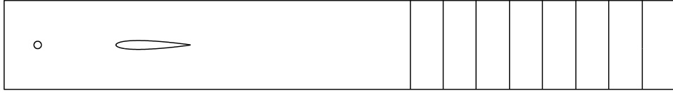
Figure 3.4: The permeable FW-H integration surface used for farfield noise prediction using the Charles simulation data. The “endcaps” remove numerical errors (expected to be uncorrelated over the end surfaces) through the integration process.
